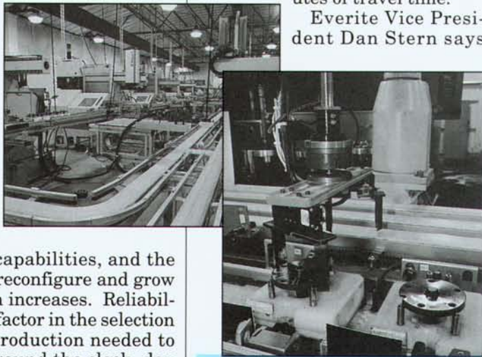
The conveyor system offers accurate pallet indexing, position sensors, accumulation capabilities, and the flexibility to reconfigure and grow as production increases. The automated pick-and-place material handling capabilities help Everite meet exacting specifications.
