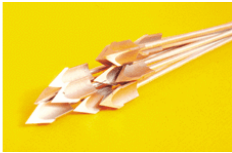
Electrochemical grinding puts an edge on these stainless steel trocars, surgical instruments used to perforate the body and drain fluids.
