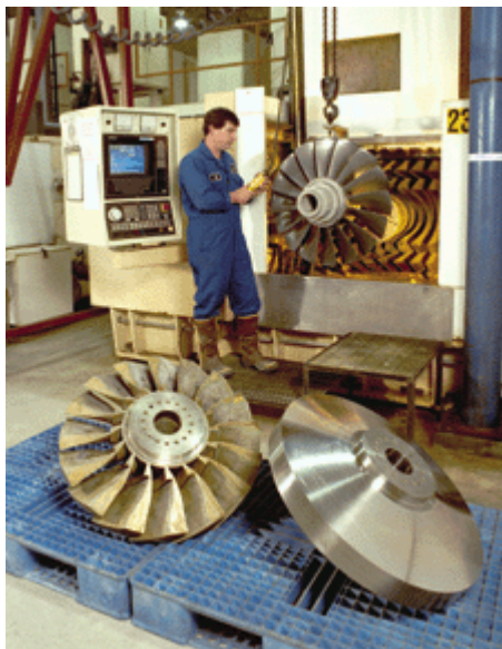
The three stages of electrochemical machining: in the foreground, a forging (right) and a rough cut; a Sermatech technician removes the finished bladed disc from an ECM unit.
